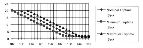
Figure 26. Overload trip time versus percent RLA
